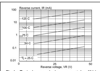
Fig.4. Typical reverse leakage current;  $I_R = f(V_R)$ ; parameter T
