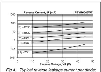
Fig.4. Typical reverse leakage current per diode;  $I_R = f(V_R)$ ; parameter  $T_i$
