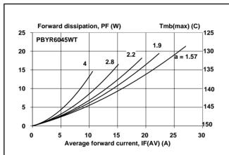
Fig.2. Maximum forward dissipation  $P_F = f(I_{F(AV)})$  per diode; sinusoidal current waveform where  $a = f(I_{F(AV)})$  $factor = I_{F(RMS)} / I_{F(AV)}$ .
