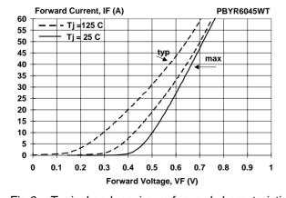
Fig.3. Typical and maximum forward characteristic  $I_F = f(V_F)$ ; parameter  $T_F$
