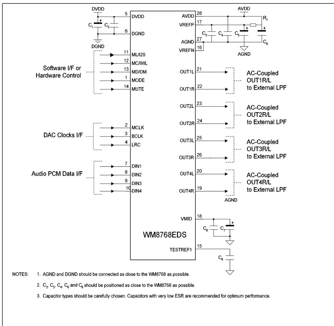
Figure 28 Recommended External Component Diagram
