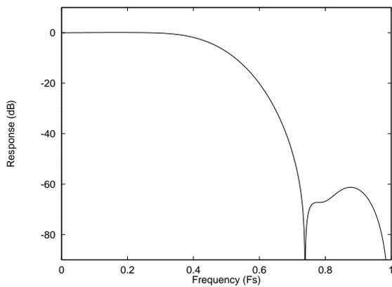
Figure 20 DAC Digital Filter Frequency Response – 192kHz
