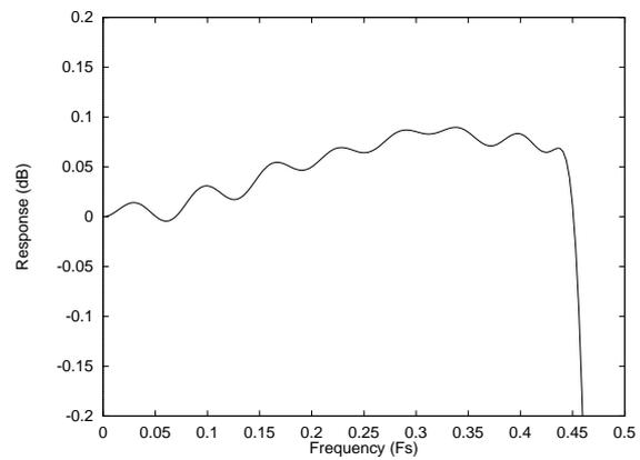
Figure 19 DAC Digital Filter Ripple – 44.1, 48 and 96kHz
