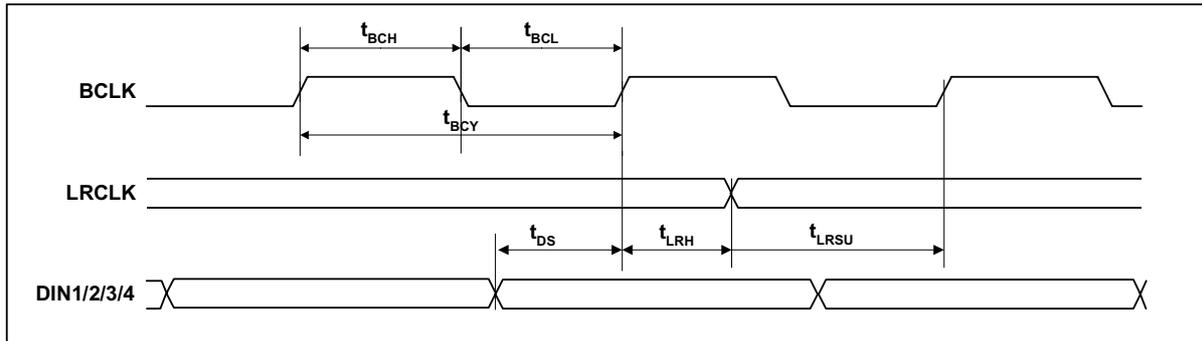
Figure 5 Digital Audio Data Timing – Slave Mode
