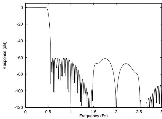
Figure 18 DAC Digital Filter Frequency Response – 44.1, 48 and 96kHz
