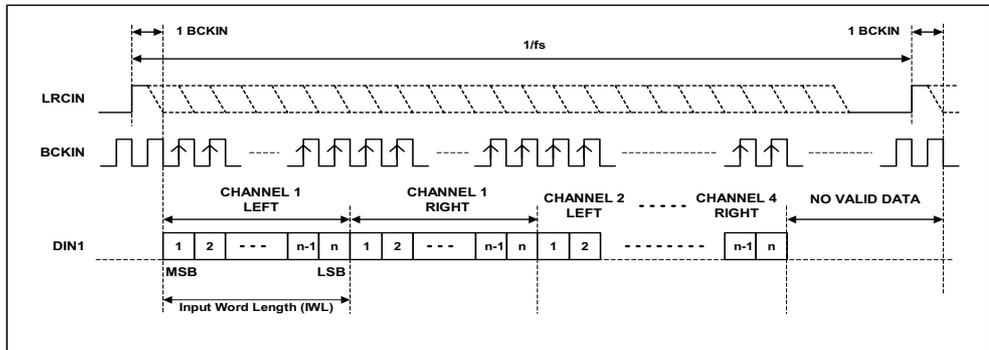
Figure 14 DSP Early Mode Timing Diagram – DAC data input
