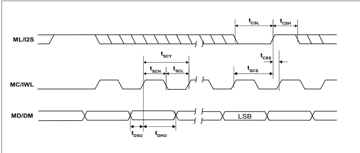
Figure 6 SPI Compatible Control Interface Input Timing
