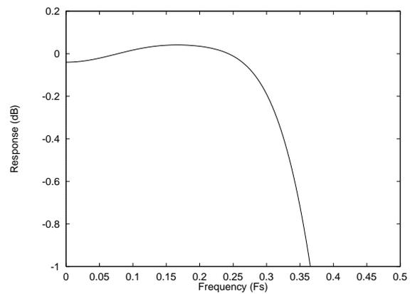
Figure 21 DAC Digital filter Ripple – 192kHz
