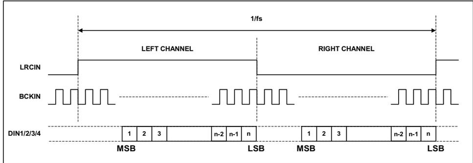
Figure 12 Right Justified Mode Timing Diagram
