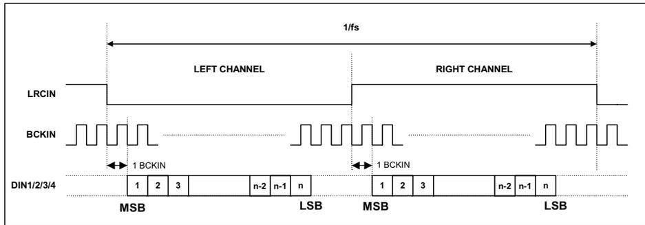
Figure 13 I<sup>2</sup>S Mode Timing Diagram
